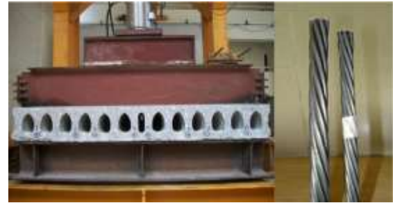
Figure 1: Details for tested PHC slabs and pre-stressing strands
