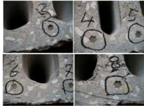
Figure 10: Anchorage failure of the eight strands in SA
